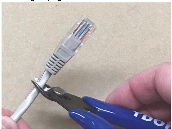
2. Using the strip blade of an Ethernet crimp/cut/strip tool remove roughly 1 inch (30 mm) of the protective sleeve
