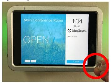
4. Tilt the paperclip until you feel the iPad power button being pressed, then hold until the power off menu appear
